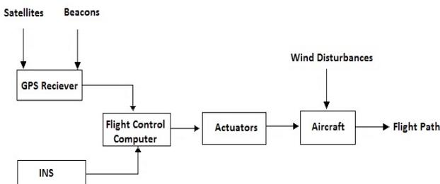
**Figure 8: System Architecture**
