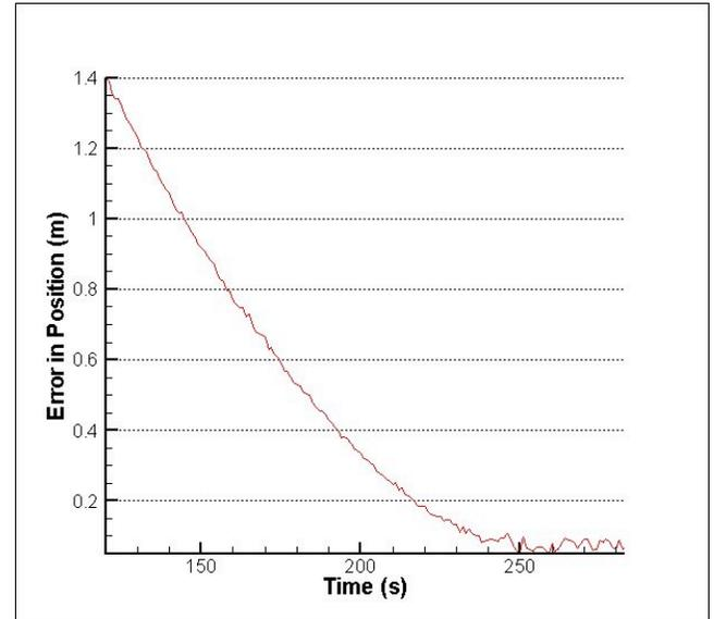
Figure 7: Error in position during CDGPS mode
