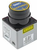
Figure 4.4: Hokuyo URG-04LX 2D Laser Scanner [8]
