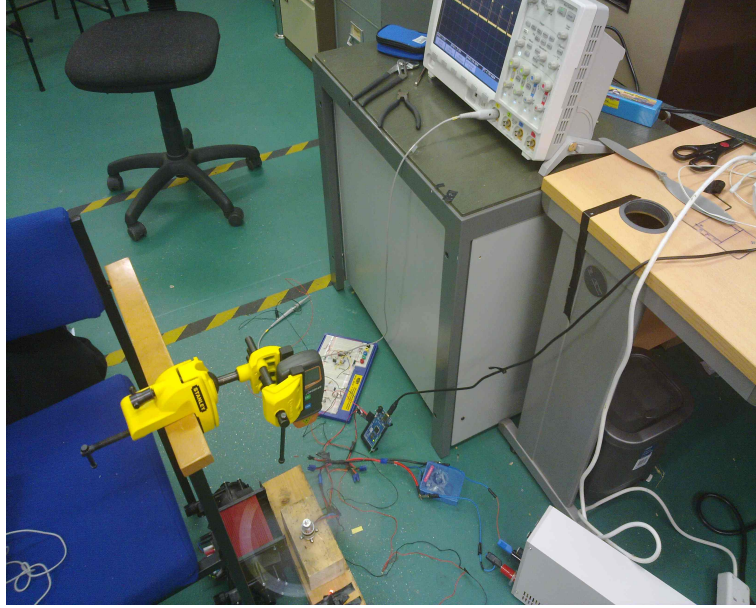
Figure 5.6: Motor dynamic response testing rig
