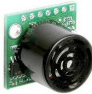
Figure 4.8: MaxSonar LV-EZ0 ultrasonic range finder
