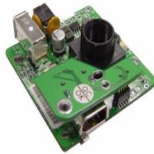
Figure 4.5: Unibrain Fire-i board camera [12]
