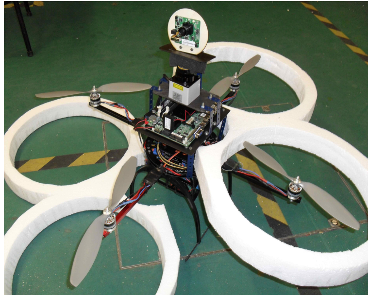
Figure 7.2: The fully assembled BumbleBee quadrotor
